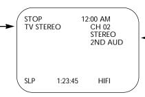
The indication 2ND AUD or STEREO that appears on this side of the status display tells you if the program you're watching is available in second audio or stereo. Even though a program is available in second audio or stereo, you still must program the VCR to receive or record the program. Follow the directions on page 39. This indication is not available during tape playback.
